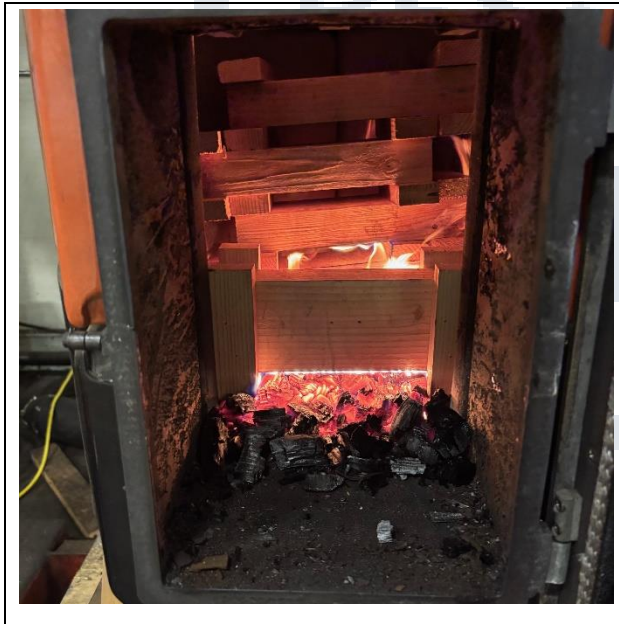
Test Fuel Loaded in Stove
