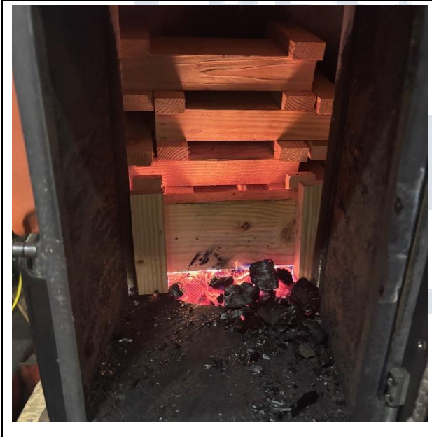
Test Fuel Loaded in Stove
