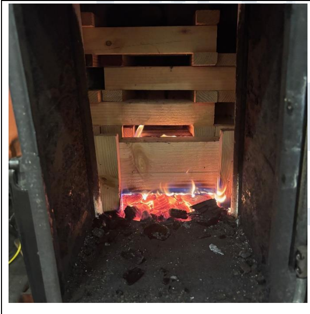
Test Fuel Loaded in Stove
